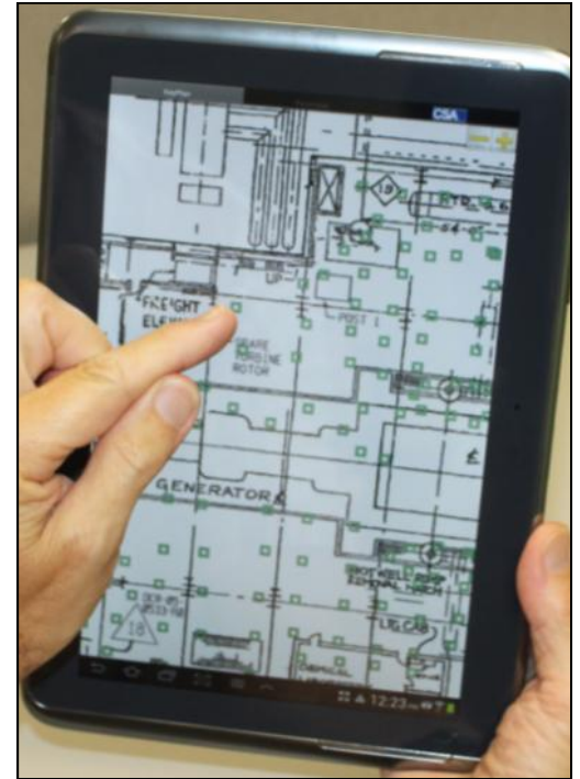
Navigate to linked 3D scans via an interactive keyplan. Green squares on map represent individual 3D scanner locations.
